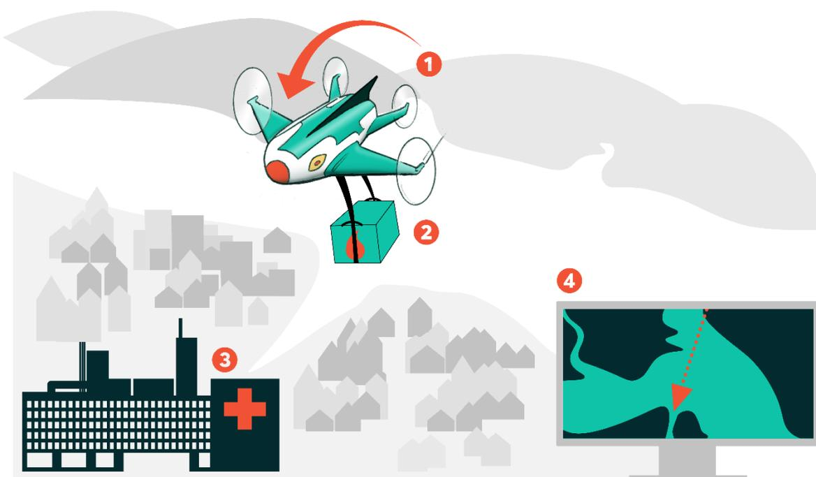
*The drone (1) takes off vertically from the mainland, having picked up a cargo of medical deliveries (2), flies over the Solent to a medical facility on the Isle of Wight (3). The flight would take place beyond visual line of sight and broadcast its position to a UTM (4).*
